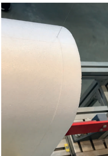
Complete channels are manufactured by means of simple cutting and gluing.
